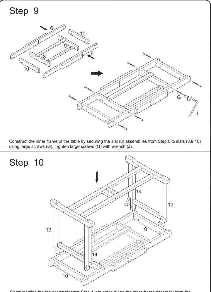
Carefully slide the leg assembly from Step 4 into place along the inner frame assembly from the previous step.
