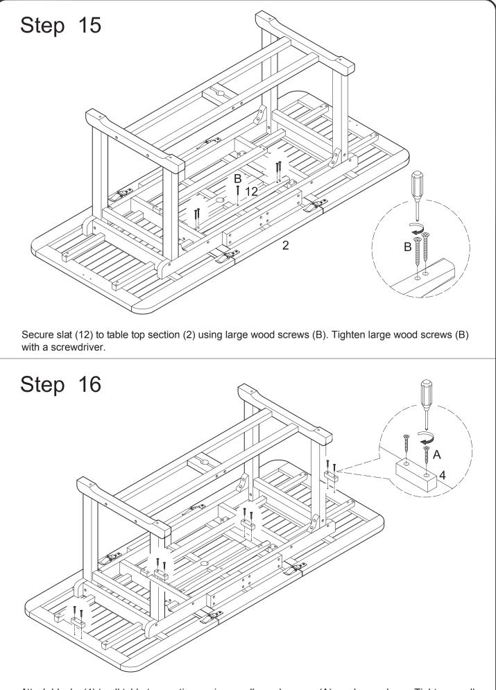
Attach blocks (4) to all table top sections using small wood screws (A) as shown above. Tighten small wood screws (A) with a screwdriver.
