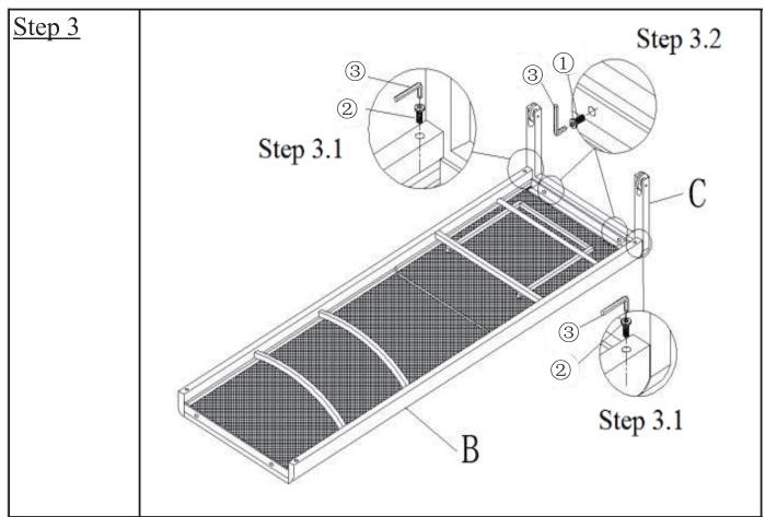
**3.1)** Attach the Back Leg(C) to the Seat Panel(B) using Bolts(2) with Allen Key(3) as shown above.
