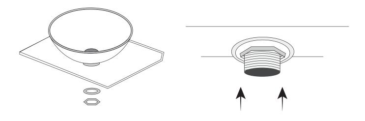
3. Put together the other half of the drain and the flexible hose. Screw off the nut on the top of the drain pipe slightly, then connect the drain and tighten it.
