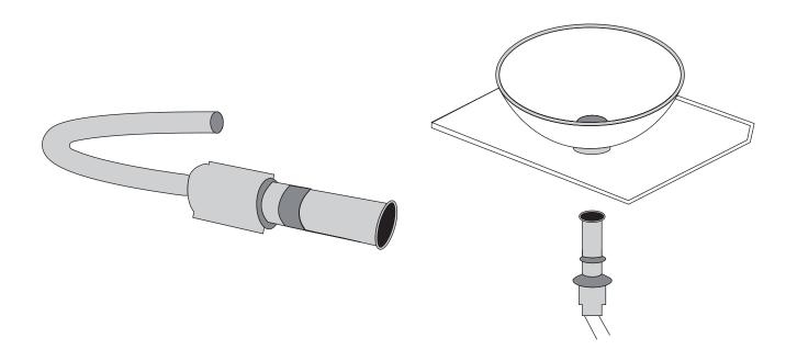
4. Connect the top half and bottom half of the drain.
