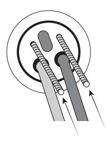
8. Put the water inlet pipe into the faucet hole of the counter, adjust the faucet to be in the correct position.
