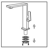
1. Remove the rubber washer, metal washer and locking nut from the faucet.
