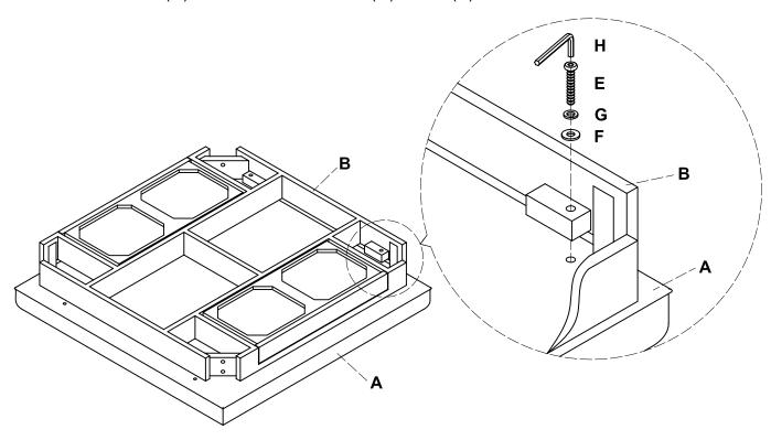
Attached Leg (**D**) to the Frame (**B**) and Bottom Panel (**C**). Use Bolt (**E**), Lock Washer (**G**), Flat Washer (**F**), on holes of Frame (**B**) and Bottom Panel (**C**). Turn the Allen Wrench (**H**) in Bolt (**E**).
