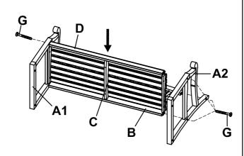
Attach the front apron (D) into seat (C) and right side frame (A1) and secure using 1 1/2" bolts (G). Next, attach the left side frame (A2) into back support (B) and front apron (D). Secure using 1 1/2" bolts (G).
