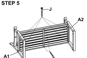
Secure the seat (C) using 1 1/2" screws (I) and 1" screws (J), as shown.
