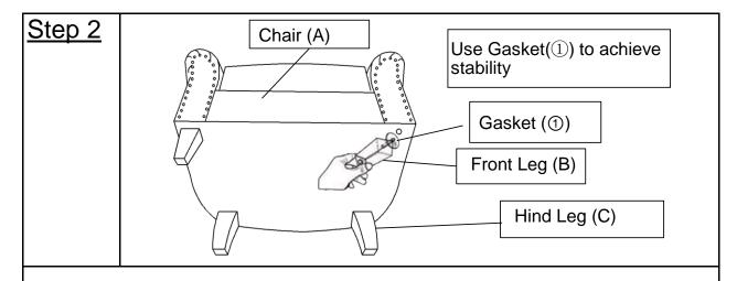
Install the first Front Leg(B) into the base of the Chair(A) by placing one Gasket(1) onto the threaded stem.
