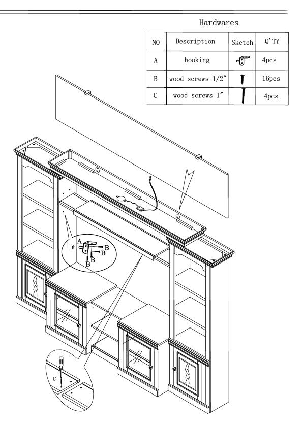
To expand shelf, remove screws, expand shelf extensions, then secure shelf extensions by reinstalling screws.
