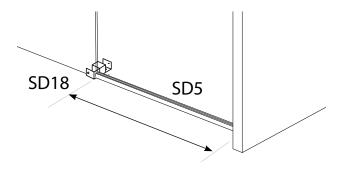
**Step 13** - Install aluminum floor strip (SD5) to prevent water leakage. Measure distance from floor bracket (SD18) to wall and cut aluminum floor strip (SD5) to fit. Put a small bead of silicone under strip for waterproofing and set in place. Tape aluminum strip to floor surface using masking tape and allow to dry for 24 hours.
