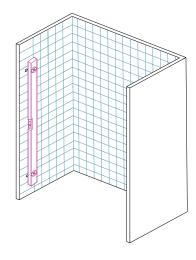
Step 2 - Measure the width of threshold tile where shower door is to be installed, this needs to be a minimum of 3" to instal this model shower enclosure. On the wall where the fixed panel is to be placed measure to the centre of the threshold tile, from here measure back toward the front of shower 1 1/8" and mark the wall with a pencil. Using a level draw a line up the wall at this point.
