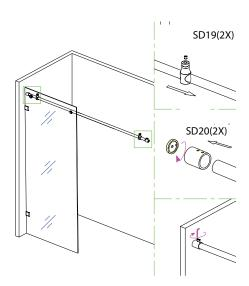
**Step 8** - Using 1/4" drill bit, drill holes and install wall plug. On one wall install only the round flat fixing piece with rest of bracket remaining on rod. On the second wall install the complete bracket. This allows you to slide the rod into one whole bracket and then screw remaining bracket on at opposing wall. Re-check the rod and glass and fixed panel are level then tighten the brackets on fix panel very tight.
