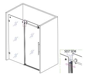
**Step 14** - Install the plastic weather strip on panels.
