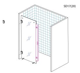
**Step 5** - Measure the width of the fixed panel and place the 1/8" thick rubber blocks provided 3" in from each end where the glass panel will sit on the tile / pan. Gently place down the glass panel on the rubber blocks & slide glass into the wall brackets. Check the glass is level, if not adjust by adding thinner 1/16" rubber block to the blocks already placed on the floor. Once level tighten the grub screws very tight on the wall brackets
