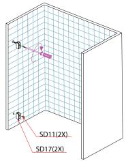
Step 4 - Install SD17 Wall Clips.
