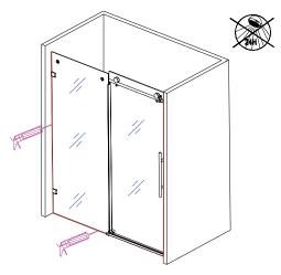
**Step 15** - Silicone the fixed panel inside and outside of enclosure.
