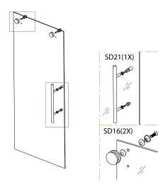
**Step 10** - Install hardware rollers and handle on door panel.
