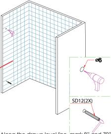
**Step 3** - Along the drawn level line, mark 8" and 70" from floor. Using a 1/4" drill bit, you will drill the holes and install the wall anchors parts SD12
