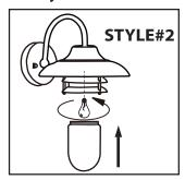
**STYLE#2** - Install proper bulb type and wattage. Unscrew glass cylinder to install bulb. Screw glass cylinder back on to the fixture.
