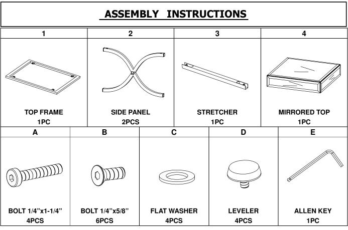
\*\*\* Do not tighten screws & bolts until the entire unit is completely assembled. \*\*\*
