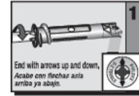
Turn E-Z Toggle into drywall until seated flush. Arrows on head indicate direction toggle clamp will open. End with arrows up and down.
