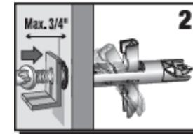
Place fixture over E-Z Toggle. Push screw into E-Z Toggle to engage clamp
