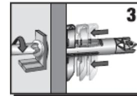
Turn screw until it stops. Toggle clamp tightens against drywall as screw is turned.
