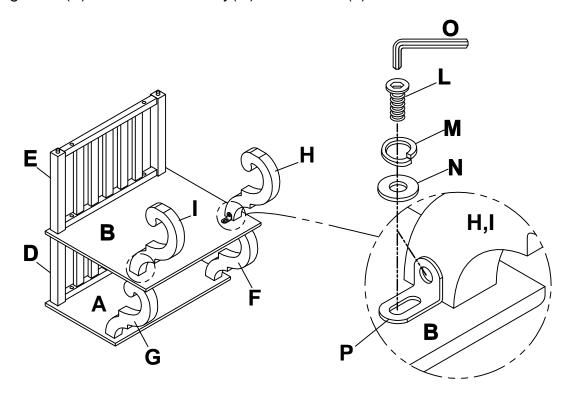
Attached Bottom(C) to the Down Back(E) and Down Post(H & I). Use Allen Bolt(K) Lock Washer(M) and Flat Washer(N) on holes of Bottom(C). Turn the Allen Key(O) in Allen Bolt(K).
