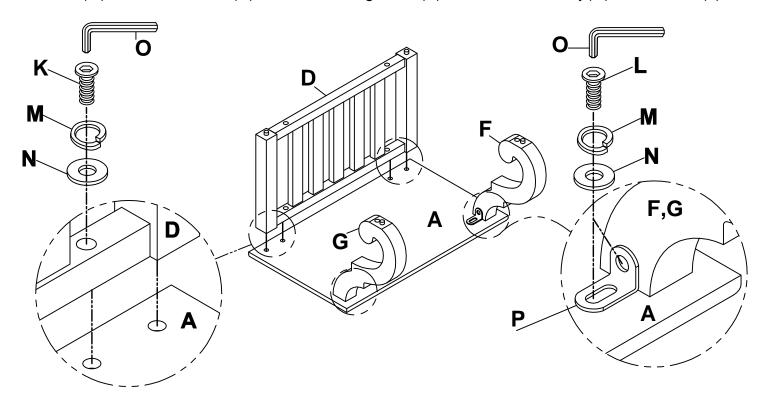
Attached Shelf(B) to the Up Back(D). Use Allen Bolt(J) Lock Washer(M) and Flat Washer(N) on holes of Down Back(E), and through holes of Shelf(B). Attached Shelf(B) to the Up Post(F & G). Use Allen Bolt(K) Lock Washer(M) and Flat Washer(N) on holes of Shelf(B). Turn the Allen Key(O) in Allen Bolt(J).
