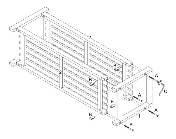
Insert Nut (B) to Part (2) ,using Bolt (A) , Hex Key( C) to secure part (1) to part (2) .
