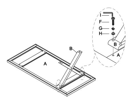
Lock a side of cross bar(C) to leg frame(B) by using flat washer(H), lock washer(G) ,bolt-large(E), allen key(I) and wooden dowel(J).
