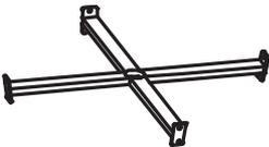
A perspective drawing of two legs crossed at their ends, connected by a central bar. | Leg Connector    | 1   |
