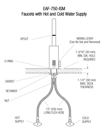
When the EAF faucet is installed on a sink that has three (3) hole punchings, a Trim Plate should be used. *Trim Plates must be specified and ordered separately:*
