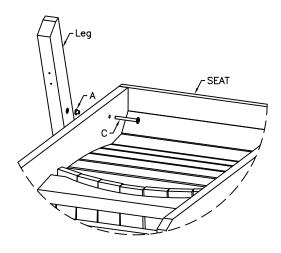
6) Turn chair over. Attach Leg to Seat using bolt C and washer A. 7) Repeat on other side.
