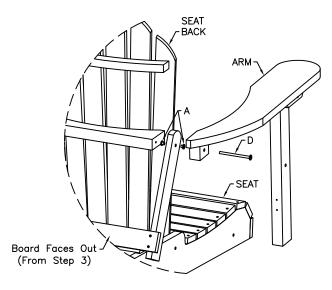
4) Attach Arm and Back Support to Back with bolt D and two A washers.
