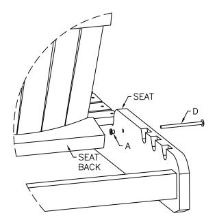
Attach seat back to seat with bolt D and washer A
