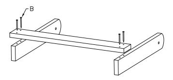
3) Attach Back Support Rail (Shorter Board) to Back Support Sides with four B screws
