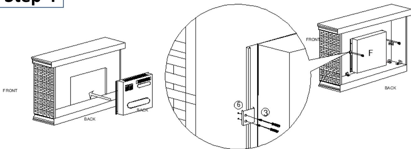
Push the fireplace insert F into the assembled part. From back side fasten the fireplace insert F to the front using 4PCS shorter srew ③ and 2PCS metal bracket ⑥ by screw driver as shown.
