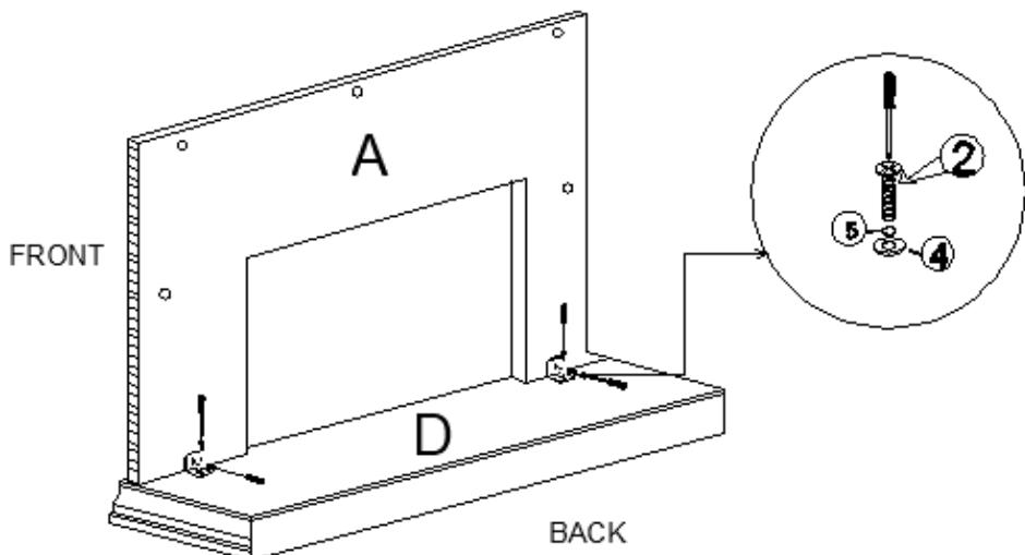
Place the wooden base D on a clean flat floor and from the back side fasten the front panel A to the wooden base D using 2pcs L brackets (1), 2pcs longer screw (2), 2pcs spring washer (5) & 2pcs flat washer (4) by screw driver **loosely**.
