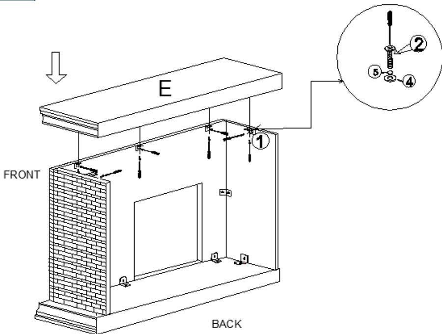
Put the wooden top E on the body and **align the front A and both side panels B&C with the front A side end to be flush with side panels by adjusting the L brackets ① or longer screw ②** and fasten the wooden top E to the body using 5pcs L brackets ① and 5pcs longer screw ②, 5pcs spring washier⑤&5pcs flat washier ④ by screw driver, and then tighten all longer screws ②.
