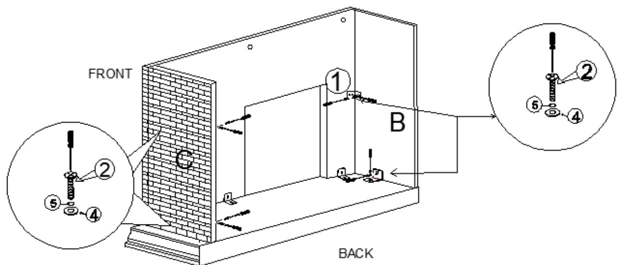
From back side fasten both side panels B&C and wooden base D using 4PCS L brackets (1), 4PCS longer screw (2), 4PCS spring washer (5)&4pcs flat washer (4) by screw driver **loosely** .**Do not tighten too much!!**
