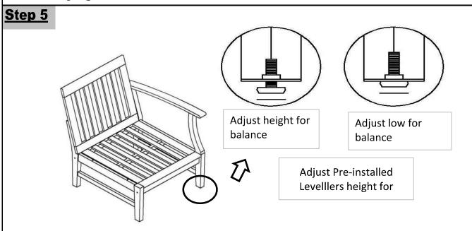
Inspect the Chair and make sure all parts are adequately connected. In a sequential manner, tighten all Bolts and Screws at all joints With assistance from your adult partners, adjust the Levellers to desired height to avoid wobbles
