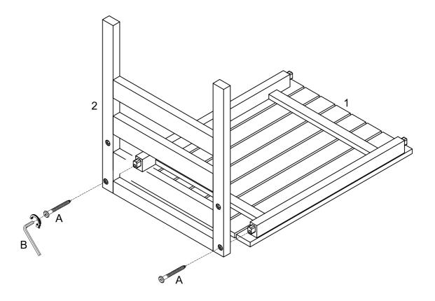
Insert bolt (A) into part (2) to part (1) with hex key (B) as per diagram.
