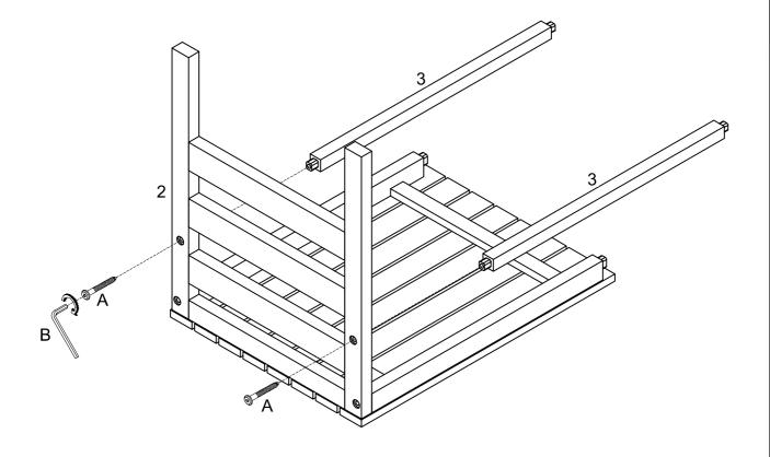
Insert bolt (A) into part (2) to part (3) with hex key (B) as per diagram.
