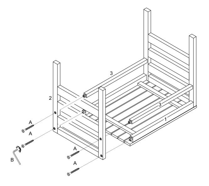
Insert bolt (A) into part (2) to part (1,3) with hex key (B) as per diagram.
