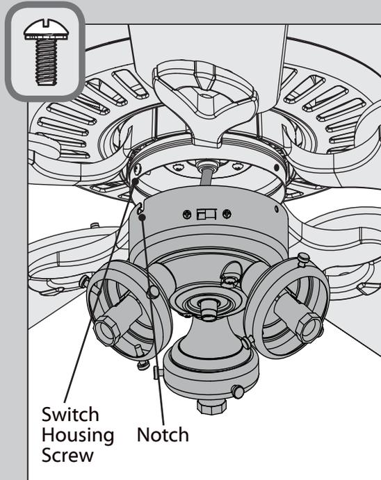
Partially install two of the switch housing screws found in the ☰ bag. Align the notches in the sides of the lower switch housing with the screws on the upper switch housing. Twist the lower switch housing clockwise to lock into place.
