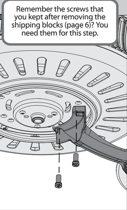
⊗ Lightly attach the blade irons to the motor with the blade iron armature screws, then securely tighten after both screws are attached.
