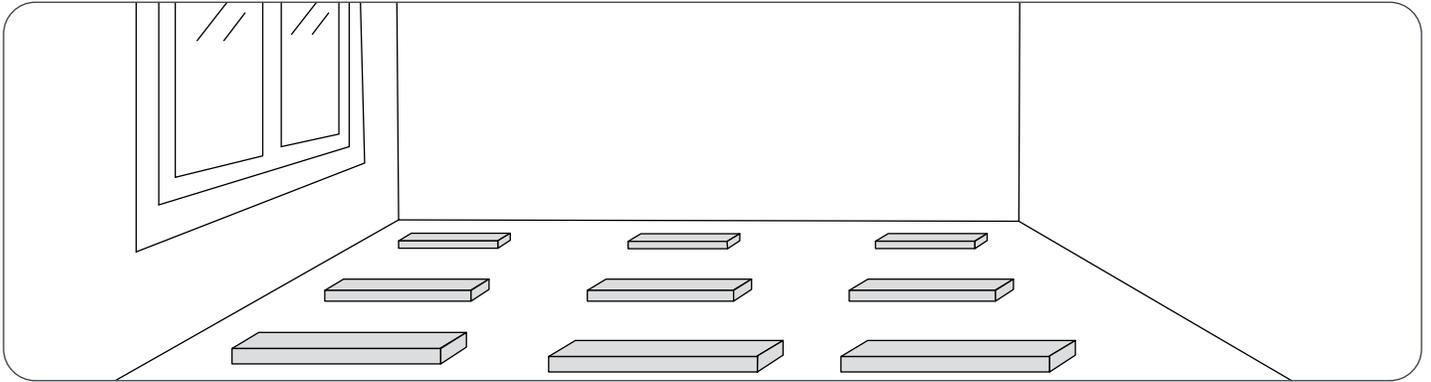
**TIP - 2 :** Cut a piece of tile/plank and use it as a tapping block.
