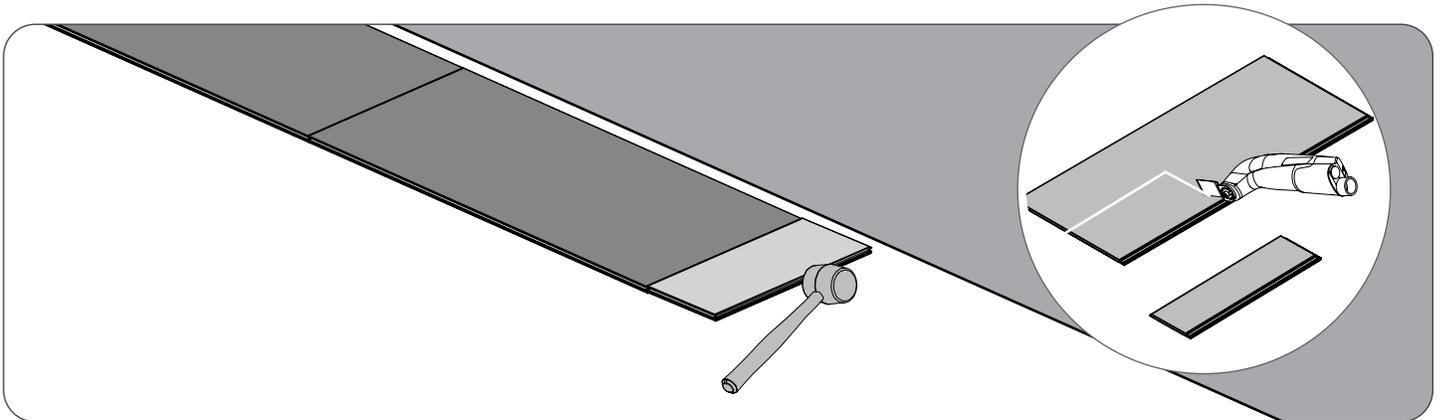
**TIP - 3 :** When installing flooring around door trims and it is challenging to use the click lock profiles, remove the top section of the click lock profile to allow you to slide in the plank or tile under the installed floor. Apply the recommended silicone , on [page 5](#), along the click lock profile and slide it under the installed flooring. Make sure to wipe off any excess glue and ensure glue used will dry in clear colour.
