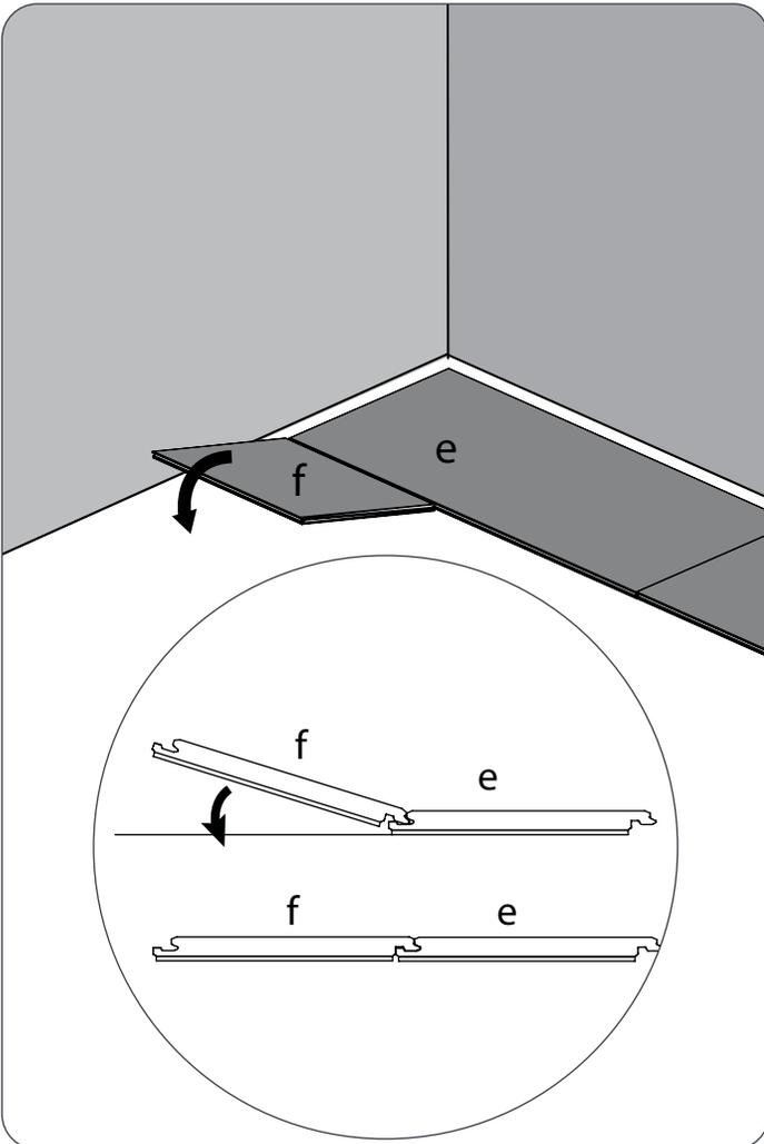
**12** Place your second tile on an angle along the long edge of the first row and drop the tile down.
