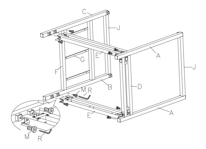
Using bolts (M) and allen wrench (R) again, attach canopy long stretcher (I) the assembled headboard and footboard as shown.
