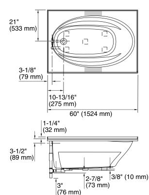
No change in measurements if connected with drain illustrated. (K-11677)
