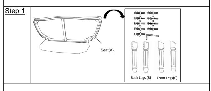
Place the Seat(A) on a clean, non-marring surface with the bottom facing you, as shown in picture above.
