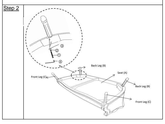
Insert one Back Leg(B) into the mounting position of Seat(A) and attach using Bolts(①), Spring Washers(②) and Washers(③) with Allen Key(④). **Do not fully tighten the Bolts.**
