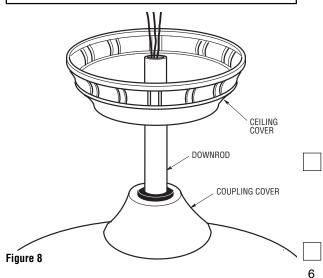
14. Make sure the grommet is properly installed in the coupling cover, then slide the coupling cover on the downrod until it rests on the motor housing. Place the ceiling cover over the downrod. Be sure that the ceiling cover and the coupling cover are both oriented correctly (Figure 9).
