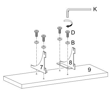
Attach shelf racks (5L,5R) to shelf crossbar (6) using large bolts (C). Build each shelf by attaching shelf supports (7,8) to shelf top (9) using small bolts (D) and washers (B).
