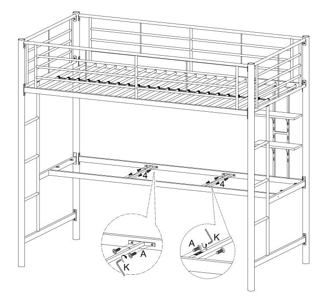
Attach desk crossbars (4) to the bunk bed frame using medium bolts (A).
