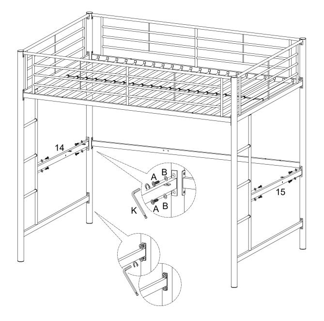
Attach crossbars (14,15) to the bunk bed frame using medium bolts (A) and washers (B). Retighten the bolts that secure the short crossbars.
