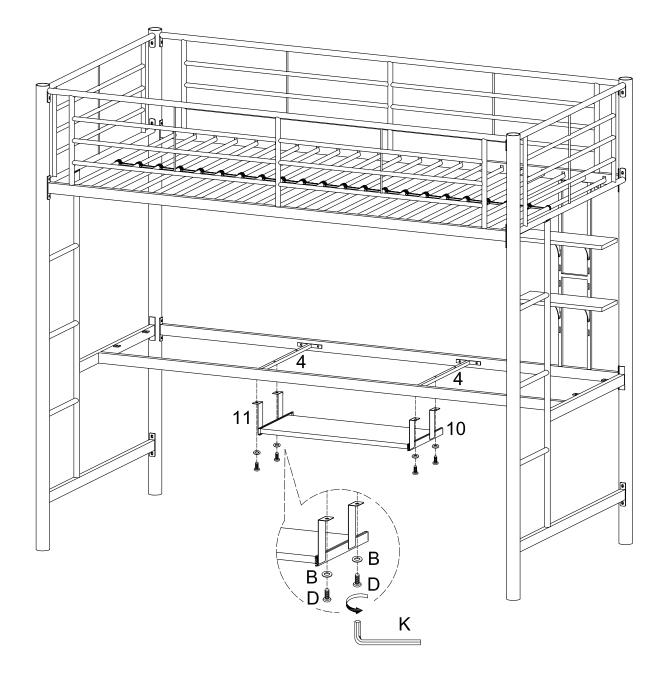
Attach the keyboard assembly from Step 10 to crossbars (4) using small bolts (D) and washers (B).
