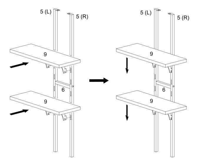
Attach the assembled shelves from Step 6 to shelf racks (5L,5R) by inserting them in at the desired height and gently pushing down to lock in place.
