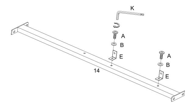
Attach angle brackets (E) to crossbars (14,15) using medium bolts (A) and washers (B).
