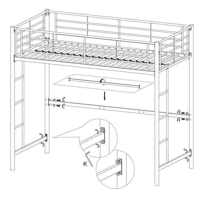
Remove the long crossbar from the bunk bed frame and turn it over so the screw holes are facing forward. Reattach the long crossbar to the bunk bed frame using the bolts and washers from Step 1. Loosen, but do not remove the bolts that anchor the short crossbars to the bunk bed frame.
