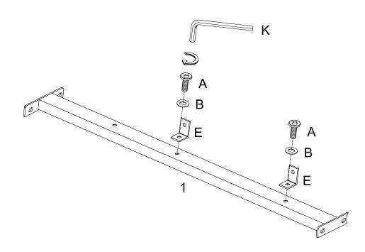
Attach angle brackets (E) to crossbars (1,2) using medium bolts (A) and washers (B).
