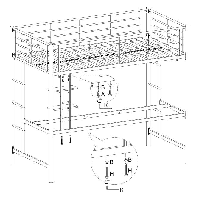
Attach the shelf assembly from Step 7 to the bunk bed frame using extra-large bolts (H) and washers (B).
