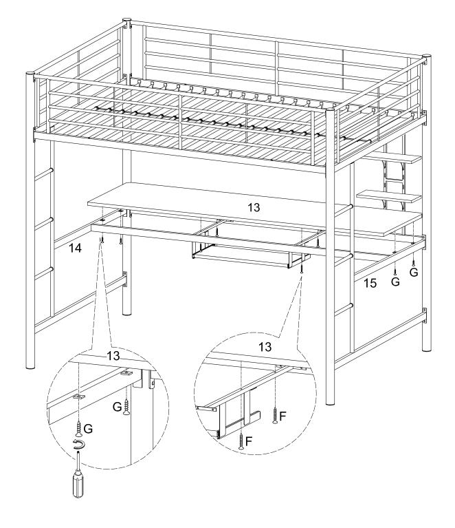
Attach the desk top (13) to the bunk bed frame using medium screws (G) on either end, and large screws (F) at the keyboard tray assembly.
