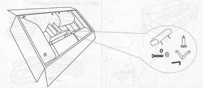
Step 1: Assemble the leg (E) onto the seat frame(A & B) with 2pcs bolt (G) by Allen wrench (D)
