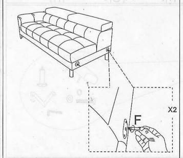
Step 4: Align the connecting bolt (F) with the accembling holes on chaise (B) to tighten sofa (A) and chaise (B) together.
