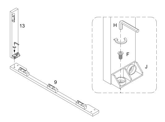
Attach plastic wedge (J) to part (9) using screw (F) with Hex key (H).
