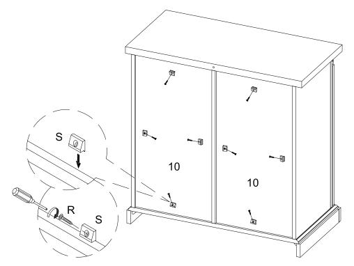
Attach plastic wedge (S) to part (10) using screw (R) with screwdriver.
