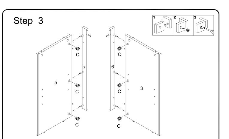
Attach part (5,3) to part (7,6), then insert and secure cam lock (C) to part (5,3) to lock it.
