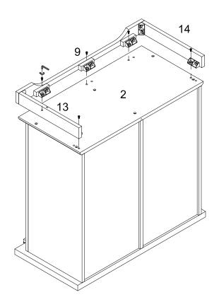
Attach part (9,14,13)to part (2) using plastic wedge(J) with hex key (H).
