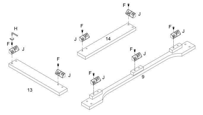
Attach plastic wedge (J) to part (13,14,9) using screw (F) with Hex key (H).
