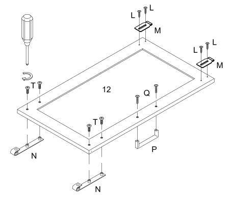
Attach pulley (N) using bolt (T), and door guide (M) using screw (L) to part (12) with screwdriver.
