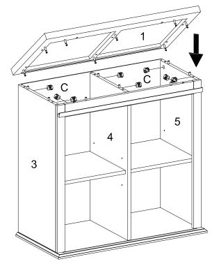
Attach part (1) to part (3,4,5), then insert and secure cam lock (C) in part (3,4,5,8) to lock it.
