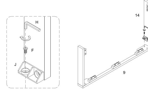
Attach plastic wedge (J) to part (9) using bolt (F) with Hex key (H).
