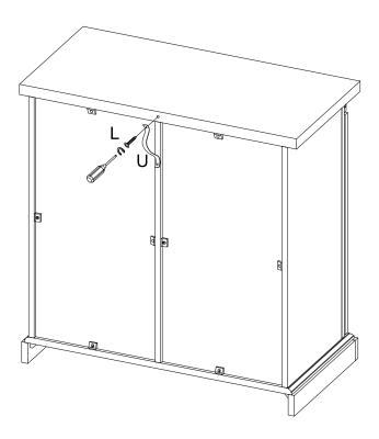
Using screwdriver to secure screw (L) with the plastic strap (U)
