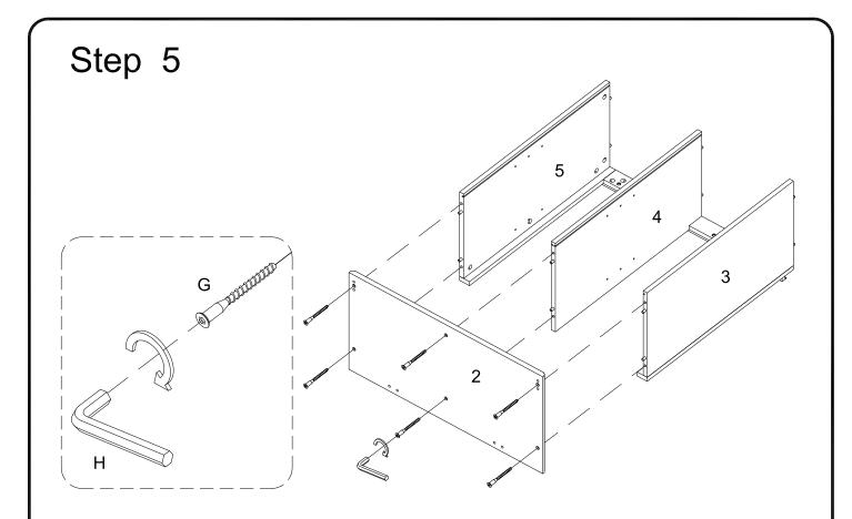
Attach part (2) to part (3,4,5) using screw(G) with hex key (H). Note: Groove for the back panel should be aligned
