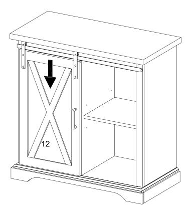
Hang pulley (N) to part (8), then press down to hold the door
