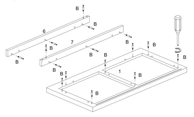
Attach cam bolt (B) to part (6,7,1) with screwdriver.
