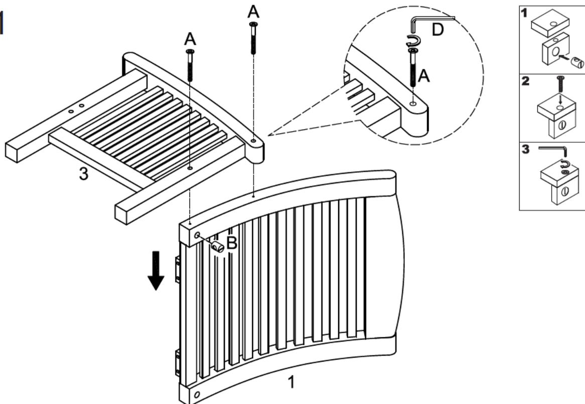
Insert barrel nuts (B) into chair back (1). Attach chair side (3) to chair back (1) using bolt (A). Bolt (A) will be inserted through chair side (3) and will screw into barrel nuts (B). Tighten bolts (A) firmly with wrench (D).
