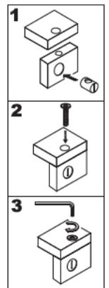
Insert barrel nuts (B) into chair seat (4). Attach chair side (4) into the chair side (2&3) using bolt (A). Bolt (A) will be insert through chair side (2&3) and will be screw into barrel nuts (B). Tighten bolts (A) firmly with wrench(D).
