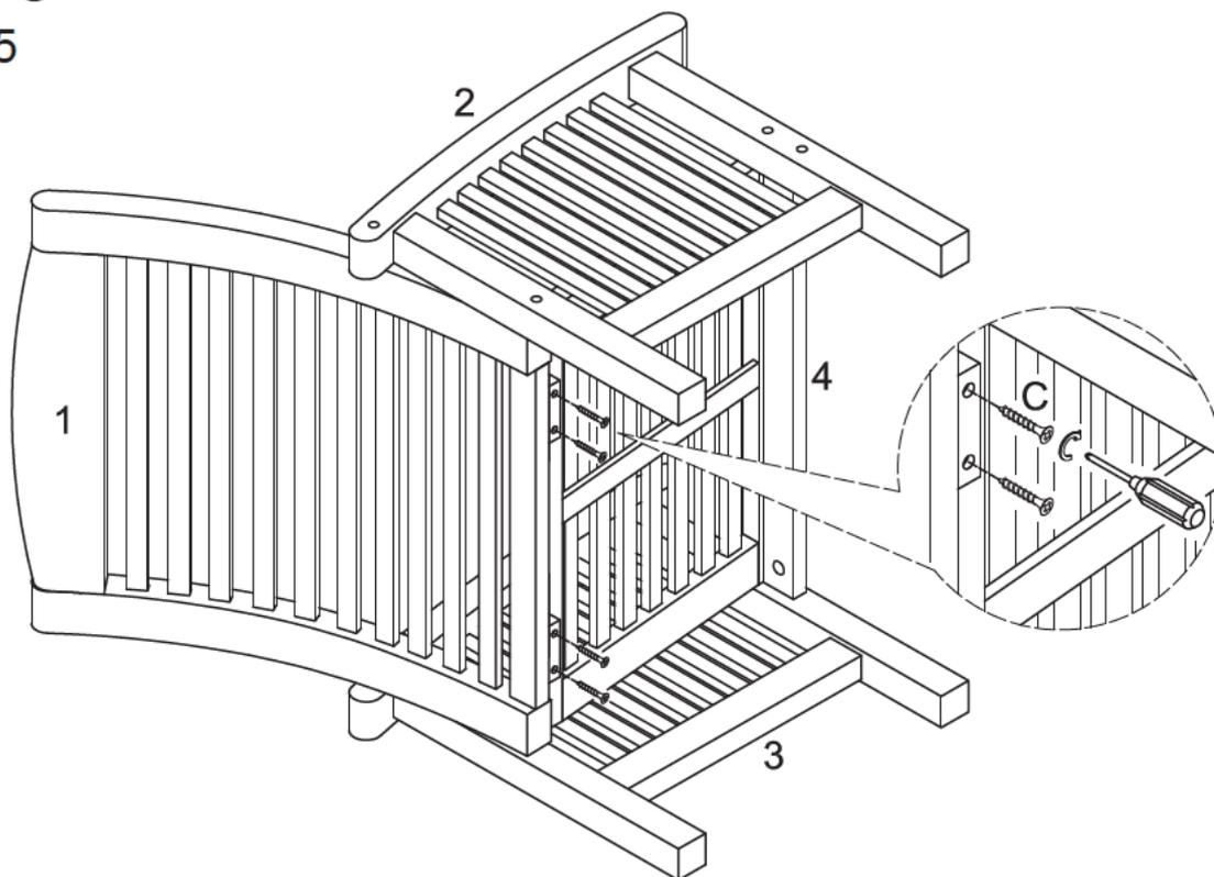
Secure chair seat (4) to chair back (1) using screws (C). Tighten screws (C) firmly with a screwdriver.
