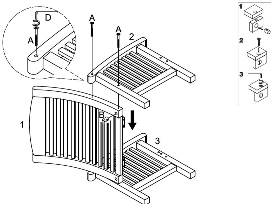
Insert barrel nuts (B) into chair back (1). Attach chair side (2) to chair back (1) using bolt (A). Bolt (A) will be inserted through chair side (2) and will screw into barrel nuts (B). Tighten bolts (A) firmly with wrench (D).
