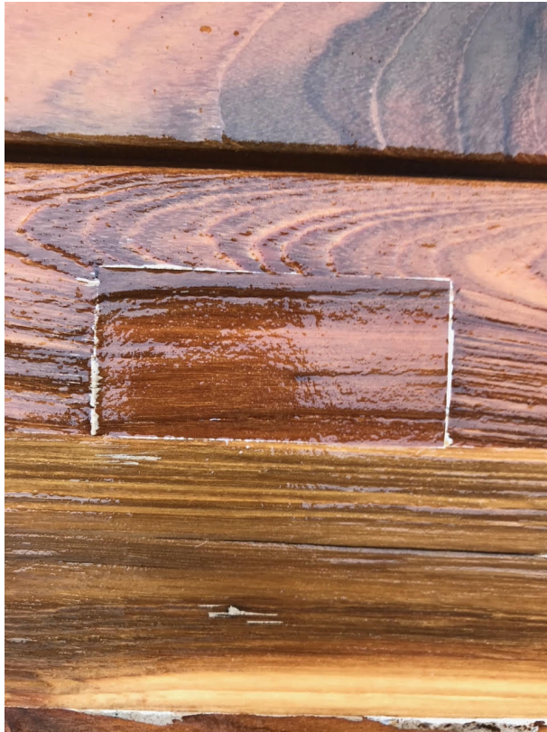
GLUE LINE AT PATCH WHEN INITIALLY WET
