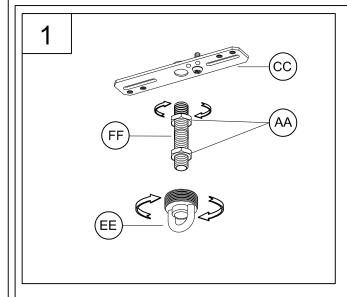
1. Screw threaded nipple (FF) into mounting strap (CC) several turns. Use one hex nut (AA) to secure parts tightly. Screw one hex nut (AA) and chain holder (EE) onto threaded nipple (FF). Tighten the hex nut against the top of the chain holder.
