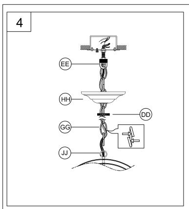
4. Pass the wires through the chain loop (JJ). Weave wires through chain (GG). Pass wires and chain through screw collar (DD) and canopy (HH). Open two links of chain and attach one end to chain loop (JJ) and the other end to chain holder (EE). Close the chain links. Pass the wires through the chain holder/threaded nipple/ mounting plate.
