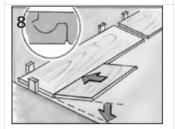
Rock and lock in half-length panel with rotating motion. Install first and second row at the same time. This will help ensure end joints are perfectly square. Planks forced down without properly engaging the tongue into the groove can result in damage.
