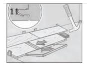
Use a 4"-6" piece to hold the tongue and groove on the same plane, limit end joint damage and ensure planks engage square. Tap end joints with multiple light taps, striking the tapping block eveny until end joints close. NOTE: Tapping too hard or striking the tapping block unevenly can result in installation-related damage or peaking.
