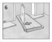
Remove the tongue on the panels that face the walls to allow room for spacers and prevent problems from spills.
