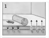
Install vapor barrier if subfloor is cement (6 mil polyethylene film).
