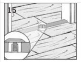
An expansion gap T-strip is required when length of planks measures 40' max and when width of planks measures 25' max. Transition strips should be placed in all doorways directly under the door when the door is closed.
