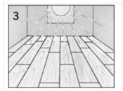
Install parallel to main light source. If no exterior light source, install parallel to longest wall.
