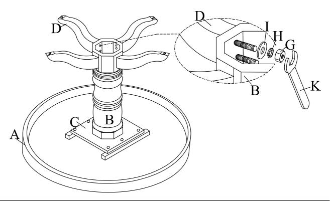
Turn the Table to upright position, place it on flat surface and adjust the Leveler so that Table is level and does not wobble. Assembly product is now completed.
