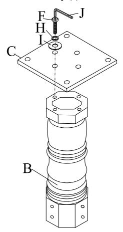
Attach the Mounting Plate (C) to Table Top (A) with Flat Washer (I), Lock Washer (H), Bolt (E) and fully tighten with Allen Key (J). Do not over tighten.
