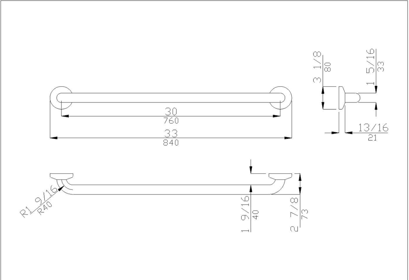
Straight grab bar, made of seamless zinc-plated steel pipe, coated with antimicrobial, biocompatible and warm-to-the-touch vinyl/PVC coated
