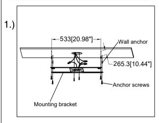
Step1.Remove mounting bracket from fixture and install to electrical box.Mark where the narrow end of the keyhole slots on the bracket meet the wall.Remove mounting bracket from wall.Drill holes using 1/4" ± drill bit where marked.Install mounting bracket to outlet box and hammer anchors into drill holes.Thread anchor screws into wall anchors until wall pate is flush with wall.
