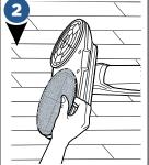
To remove mop pads, simply pull pads off the hook and loop material on the bottom of the machine.
