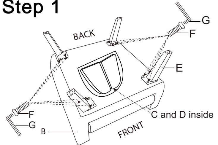
Each screw is rotated to 30% first, and the three screws on each foot are screwed in, and then completely tightened with the allen key.
