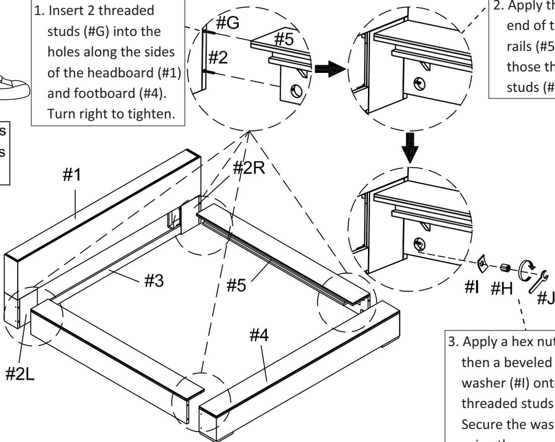
3. Apply a hex nut (#H) then a beveled washer (#I) onto the threaded studs (#G). Secure the washer using the wrench (#J).
