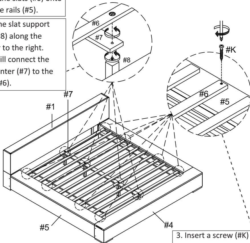
3. Insert a screw (#K) into the ends of the slats (#6). Secure using the Phillips screwdriver.
