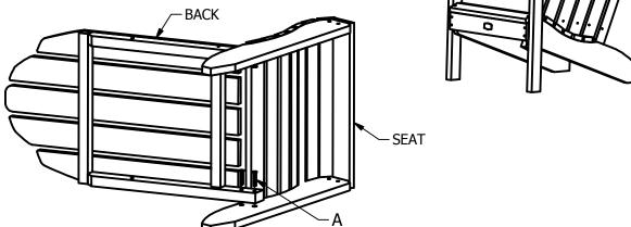
1) With the Back and Seat on their sides, attach one side of the Back to the Seat using two A bolts.
