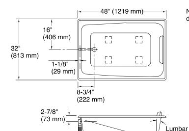
No change in measurement if connected with drain illustrated. (K-7265)
