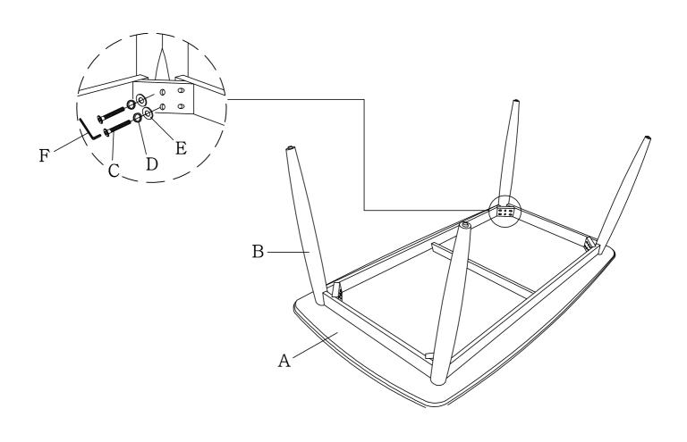
Stand table up on an even surface and check that it is balanced. If there is a slight wobble, apply downward pressure in the corner where a leg is uneven. Keeping pressure in that corner, tighten all bolts. If balanced, apply downward pressure evenly in the center and tighten all bolts. Do not over-tighten beyond hole depth.
