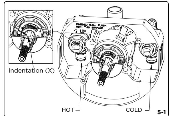
**5-2** For back to back installation, remove the base nut and remove and temperature limiting device. Turn the valve stem 180 degrees so that the indentation on the valve stem face downwards. Replace the temperature limiting device and the base nut.
