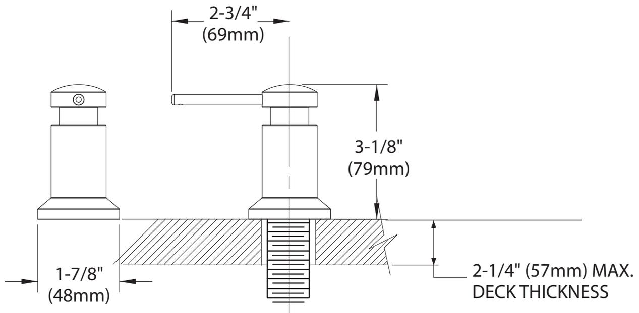
**NOTE:** DESIGNED TO BE INSTALLED THROUGH 1 HOLE 1-1/8" DIAMETER
