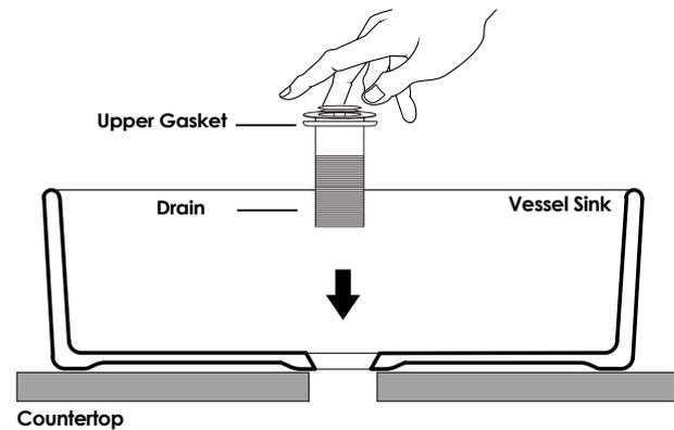
Introduce drain including upper gasket from the upper side of the sink.
