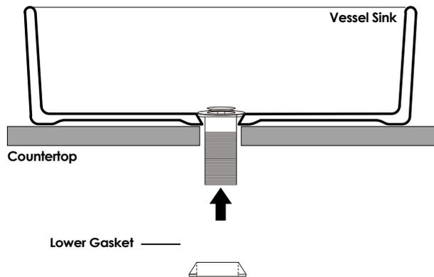
From underneath the countertop, insert lower gasket on the threaded area of the drain, it is recommended to use a Teflon layer on the threaded area in contact with mounting nut.
