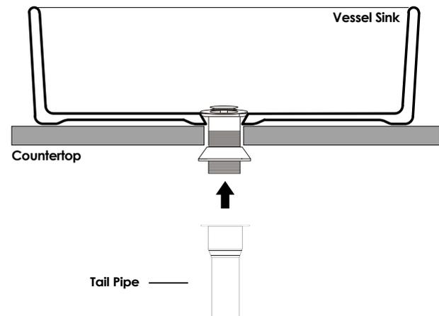
Secure the tail pipe, ensure the correct position of the black gasket, this tail pipe fits 1-1/4 inch home plumbing piping.
