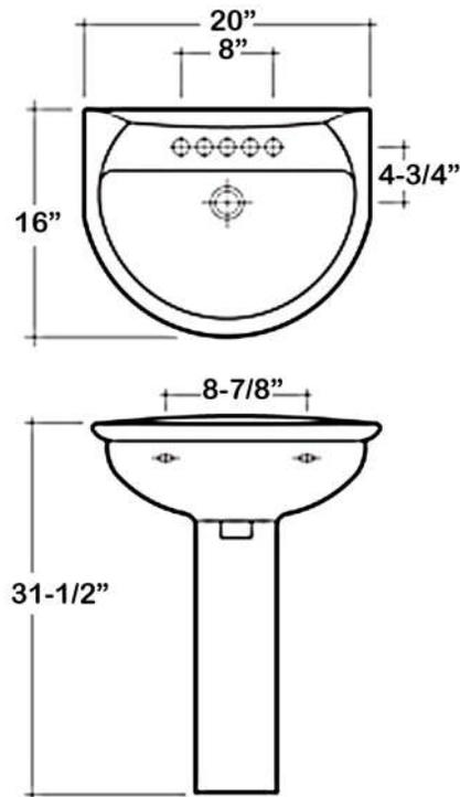
Dimensions of fixture are nominal and may vary within the range of tolerances established by ASME Standard A112.19.2-2013. Dimensions and specifications subject to change without notice.
