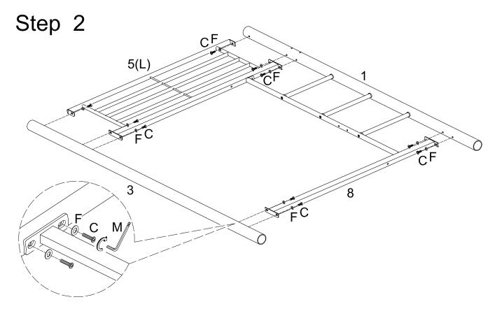
Attach guardrail (5L) and crossbar (8) to post (1) using small bolts (C) and small washers (F). Attach post (3) to guardrail (5L) and crossbar (8) using small bolts (C) and small washers (F). Tighten small bolts (C) with small wrench (M).
