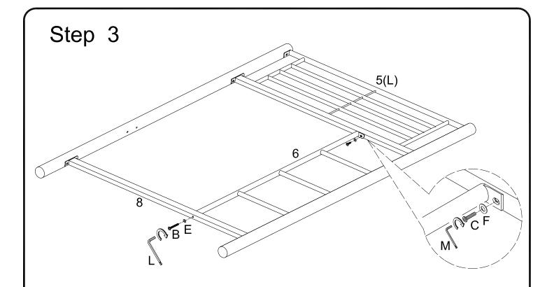
Secure ladder rail (6) to guardrail (5L) using small bolt (C) and small washer (F). Secure ladder rail (6) to crossbar (8) using large bolt (B) and large washer (E). Tighten small bolt (C) with small wrench (M) and large bolt (B) with large wrench (L).
