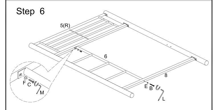
Secure ladder rail (6) to guardrail (5R) using small bolt (C) and small washer (F). Secure ladder rail (6) to crossbar (8) using large bolt (B) and large washer (E). Tighten small bolt (C) with small wrench (M) and large bolt (B) with large wrench (L).
