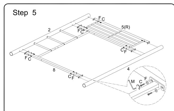
Attach guardrail (5R) and crossbar (8) to post (2) using small bolts (C) and small washers (F). Attach post (4) to guardrail (5R) and crossbar (8) using small bolts (C) and small washers (F). Tighten small bolts (C) with small wrench (M).
