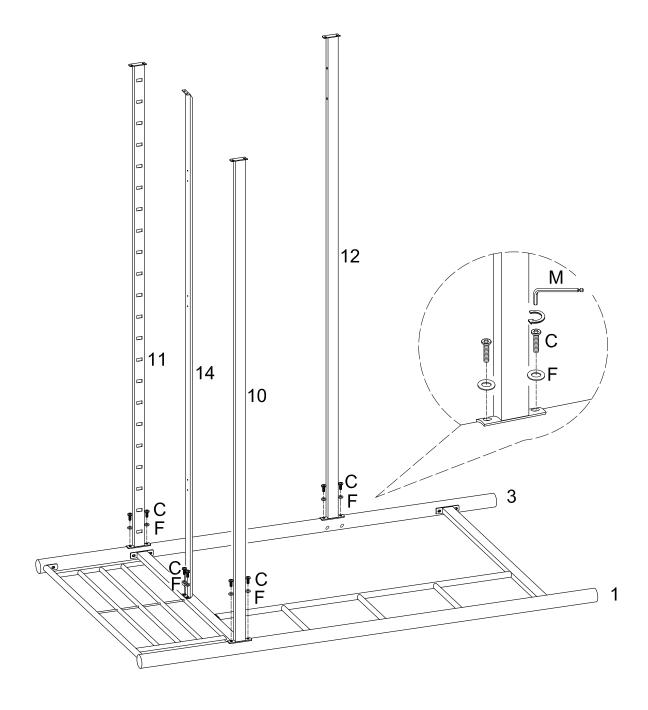
Attach crossbars (10,11,12,14) to the assembly from Step 3 using small bolts (C) and small washers (F) . Tighten small bolts (C) with small wrench (M).
