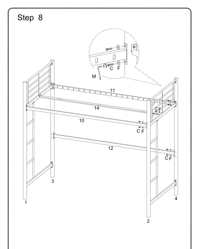
Attach crossbars (10,11,12,14) to the assembly from Step 6 using small bolts (C) and small washers (F) .Tighten small bolts (C) with small wrench (M).
