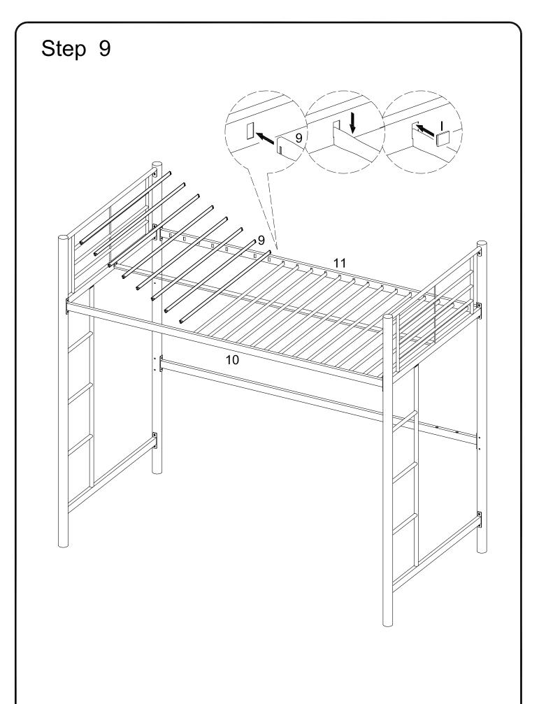
Insert mattress support bars (9) into the provoded slots of crossbars (10,11). Secure mattress support bars (9) by snapping plastic tab locks (I) into the provided slots of crossbars (10,11). Note that it may be necessary to apply more pressure to some plastic tab locks than others.
