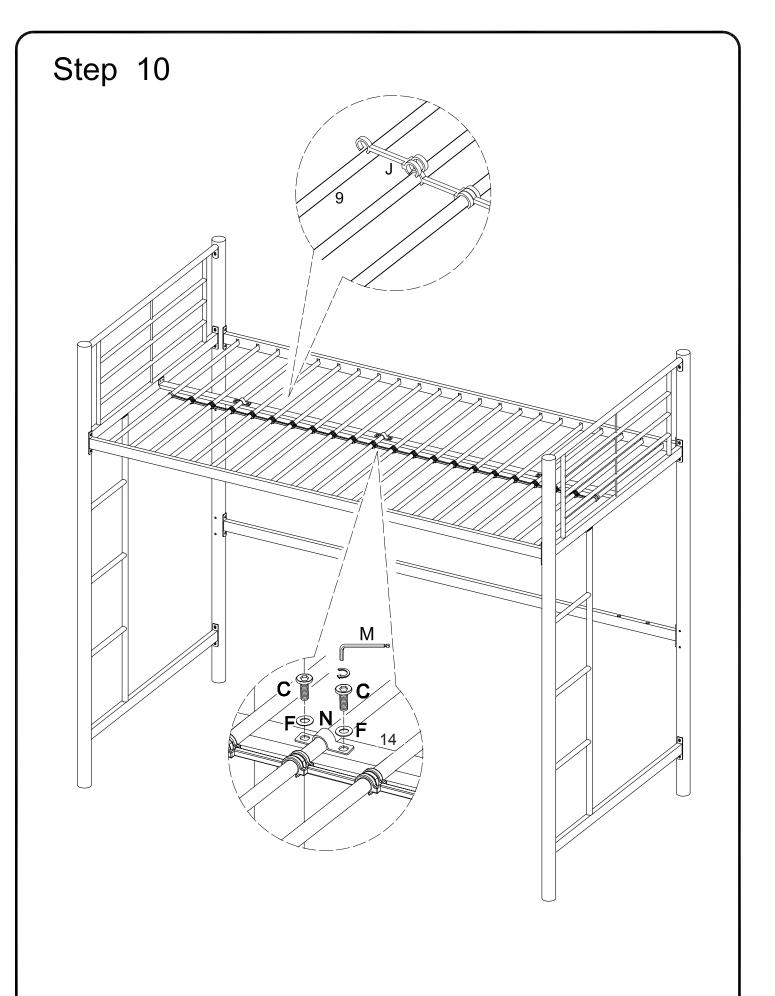
Snap plastic links (J) onto the middle of mattress support bars (9). Attach angle bracket (N) to crossbar (14) using small bolts (C) and small washers (F) . Tighten small bolts (C) with small wrench (M).
