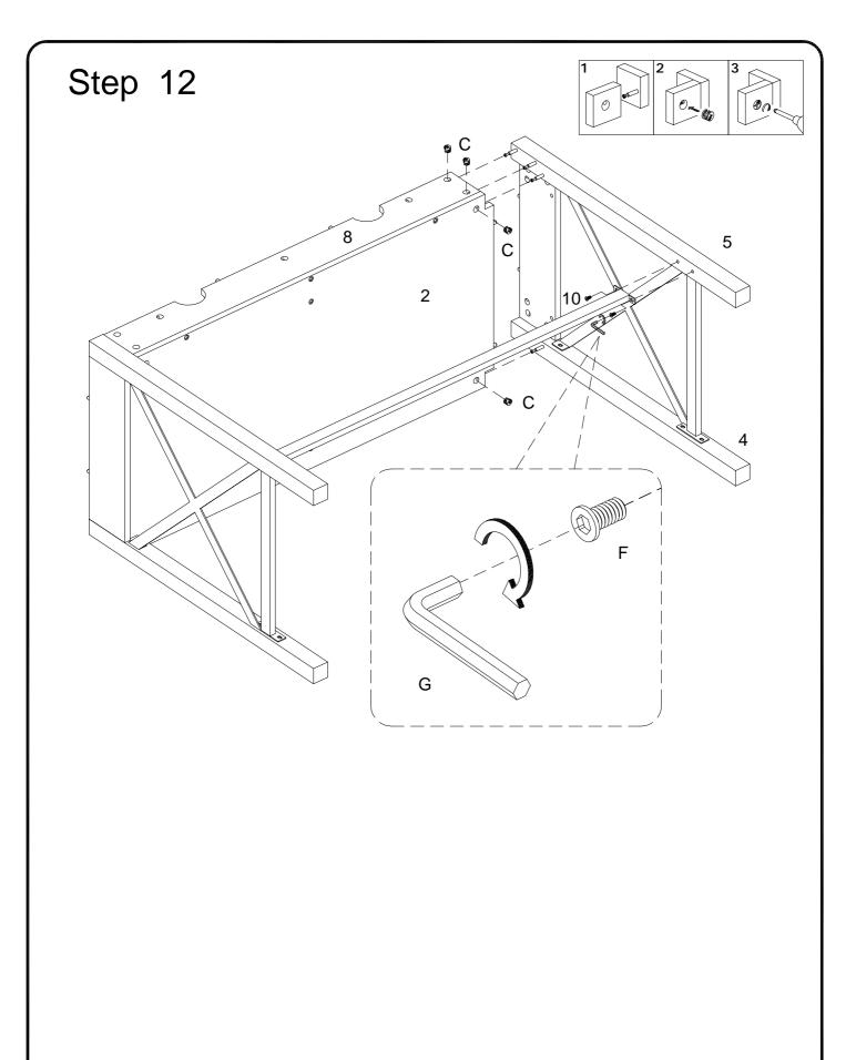
Using bolt (F) attach part (4,5) onto parts (2,8,10) and cam lock C per diagram .
