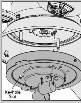
Align the three keyhole slots in the light kit with the three assembly screws in the posts. Lift the light kit and twist clockwise to lock it into place. Be sure that both pull chains are hanging freely.
