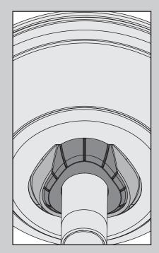
Position the canopy so that, when lifted into place, the canopy fits into the hanging bracket as shown.
