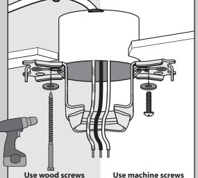
(included) when securing to support structure with approved electrical outlet box. Drill 9/64" pilot holes in support structure to aid in securing ceiling bracket with hardware found in the hardware bag.
