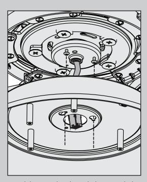
Feed the wire plug through the center hole of the upper switch housing, then wrap keyhole slots around the two screws and twist counterclockwise to lock the upper switch housing into place.
