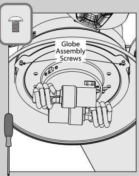
Partially install two globe assembly screws, found in the = hardware bag, halfway into the light kit assembly as shown. It does not matter which two screw holes you choose.
