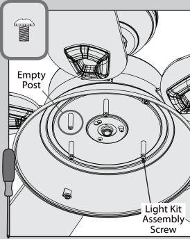
Partially install three light kit assembly screws, found in the = hardware bag, into the posts as shown, leaving the circled post empty.
