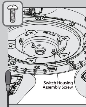
Partially install two switch housing assembly screws ,found in the = hardware bag, into the motor housing as shown. It does not matter which two screw holes you choose.
