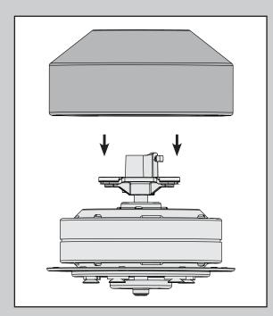
Gently lower the motor housing so it rests in place on the motor assembly.
