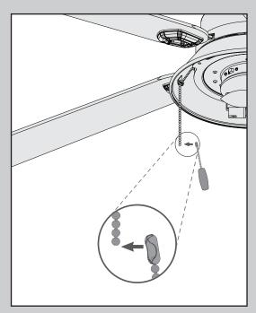
Feed the pull chains from the fan switch and the light switch down through the holes in the upper switch housing as shown. Attach the pull chain pendants to the light and fan pull chains. The fan pull chain controls the speed: from high to off. The light pull chain controls the light fixture: on and off.
