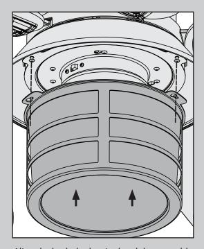
Align the keyhole slots in the globe assembly with the partially installed screws in the light kit assembly. Lift the globe assembly and twist counterclockwise to lock it into place.
