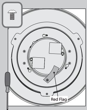
Remove the pre-installed light kit assembly screw and red flag from the light kit assembly. Save the screw. It will be needed for light kit installation.
