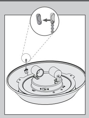
Remove and discard the plastic connectors from the ends of the two pull chains.
