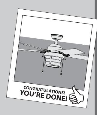
Make sure the globe assembly is securely attached to the switch housing. Failure to properly secure all three assembly screws could result in the light fixture falling.
