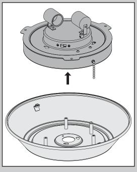
Carefully remove the light kit from the upper switch housing and set the light kit aside.
